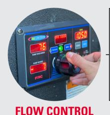
FRC pressure governors use state-of-the-art programmable microprocessor technology which operates in one of two modes, pressure or RPM. It maintains a steady pump discharge pressure and provides safety for the firefighter by controlling the engine speed or holding a selected engine RPM.
