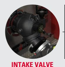
In order to deliver water to the fire scene it must first get into the pump. Intake devices are designed to bleed off air and provide protection, its important to make sure your intake appliance does not restrict flow. The Elkhart XD Intake provides unrestricted flow with only 2 psi of pressure loss at 2,000 gpm on the low profile configuration, and a large push/pull pressure-balanced bleeder valve for efficient operation.
