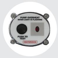
When water is not moving water through the pump and out of a discharge the water can heat up which can be detrimental to the life of the pump. A thermal protection system should be specified on all apparatus, some systems only provide an indication that the temperature is high and rely on the operator to correct the issue, while advanced systems will open a small discharge to move water through and out of the pump.
